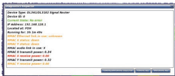
Typical PRO Series Diagnostics Inspector window with the 'ignore' buttons at the lower right corner
