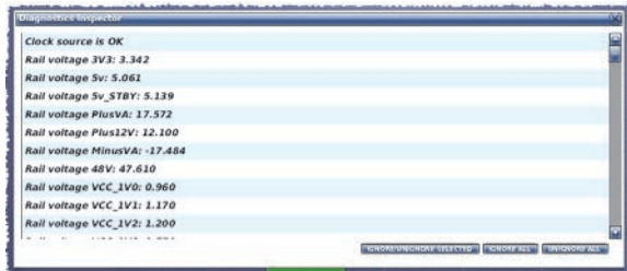
An example of DL271 DSP Board Diagnostics screen
